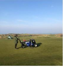
Guy with our own Air2G2 machine on 5th Green injecting compressed air into the root zone.
