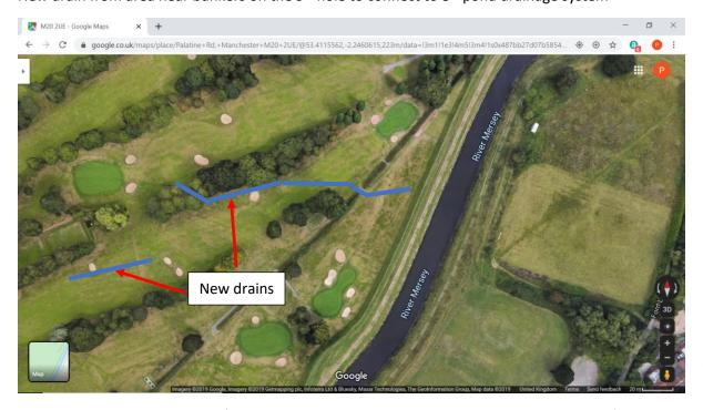
Extend land drains from the 10<sup>th</sup> hole to existing drainage on 7th, this leads into pond at 8<sup>th</sup>.
