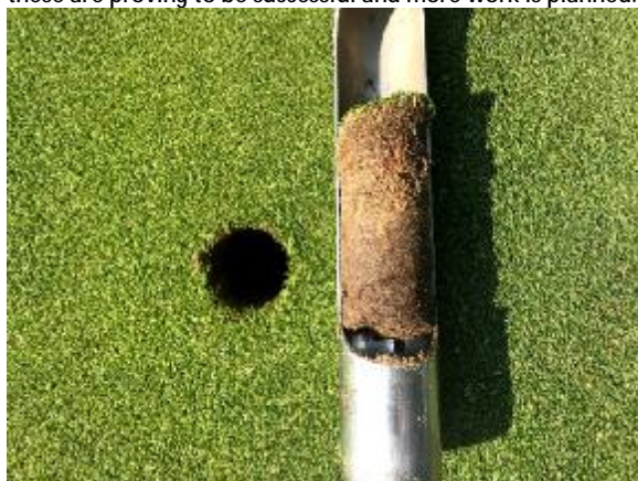
Figure 10: Soil profile conditions beneath all greens including the 10 th green shown here had the build up of organic matter in the immediate base of the turf. This should be addressed through the planned August Maintenance Week work to include verti-draining, Graden scarifying and sand dressing.
