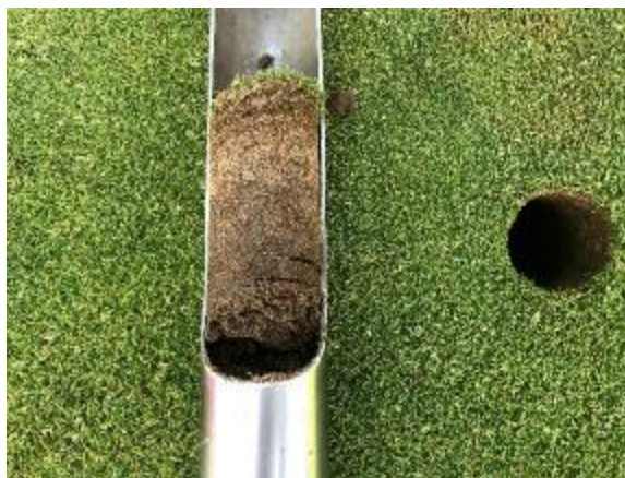
Figure 2: Soil profiles remain friable due to a combination of Toro Procore aeration and use of the Air2G2. There is however a build up of organic matter in the immediate 0-10 mm which needs to be physically removed and diluted.
