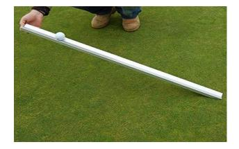
The "stimp" or "stimp rating" of a <u>putting green</u> is a numerical value that represents how fast the golf ball rolls on the putting surface. Golfers call this rating the green speed. That value is based on a measurement taken with a simple instrument called a <u>Stimpmeter</u> (hence the terms stimp and stimp rating).
