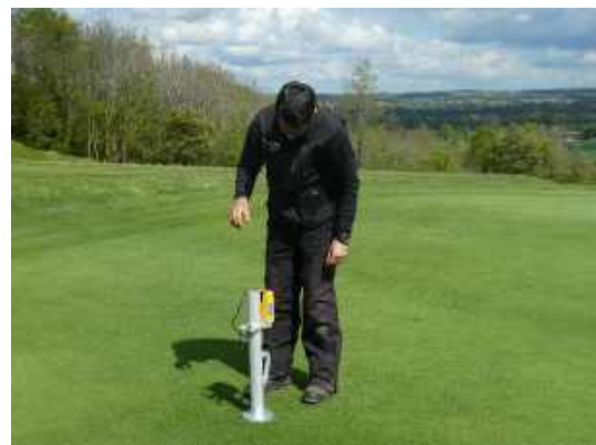
Figure 7 Testing for green firmness using a Clegg Hammer, which provides, within and between greens, measures of variability
