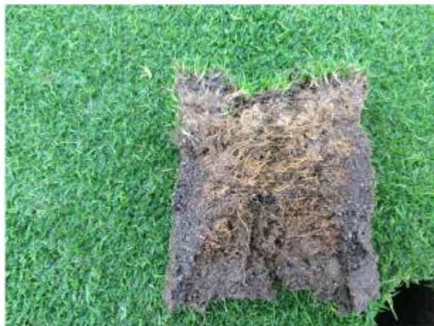
Figure 8: Thatch build up was evident beneath every green and was almost identical even beneath the sandier USGA style constructions as seen here beneath the 7 th green.
