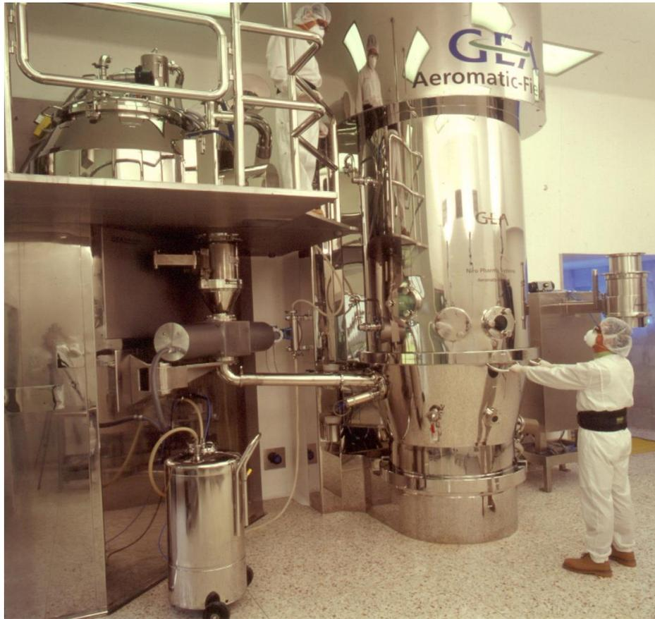
High Shear Mixer and Fluid Bed Drier Production Plant
