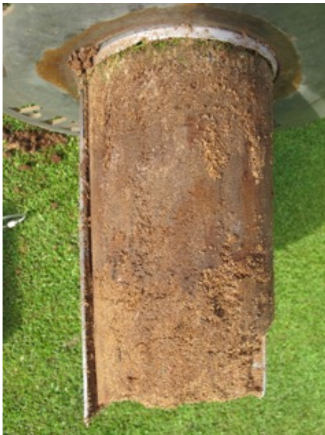
Figure 4. Soil profile from 4 th green (typical of the 'rootzone' greens)
