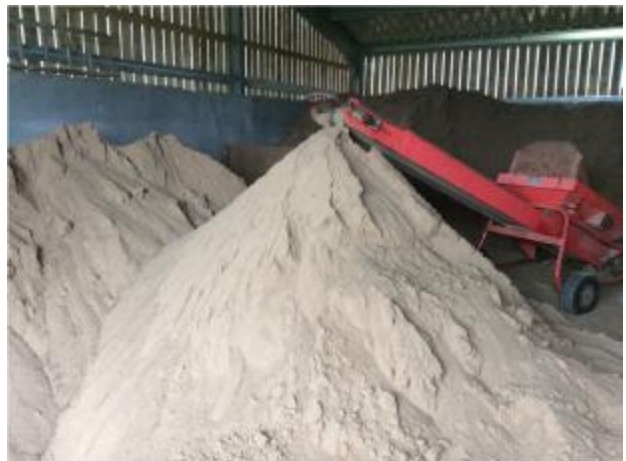
Figure 10: Locally sourced sand is screened and stored onsite, providing an excellent topdressing material.
