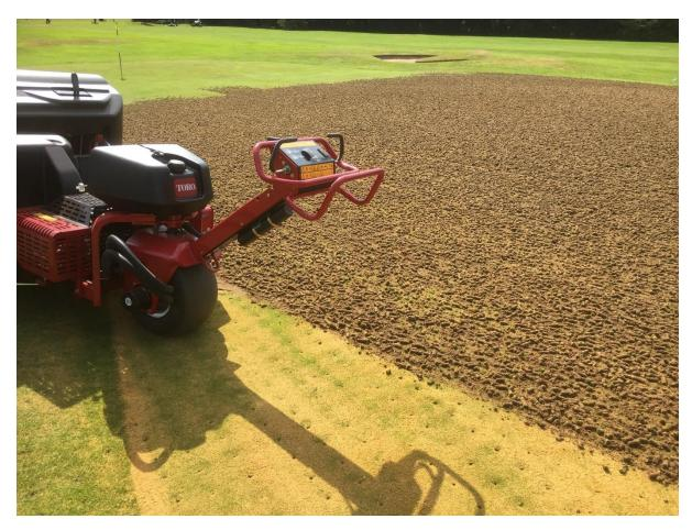
**Stage 2:** Is to verti-drain the surface with a 1" solid tine to 12" deep at 4" spacing.
