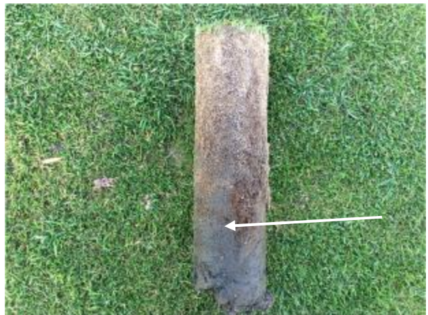
Figure 4: The 13 th green remains one of the weakest on the course and much of this can be linked to its poor drainage performance in winter. When assessing the soil profile beneath, we can see that topsoil depth is shallow and so the indigenous clay soils are closer to the surface (arrow). These hinder water movement through the soil and the introduction of pipe drainage would be the most appropriate solution.
