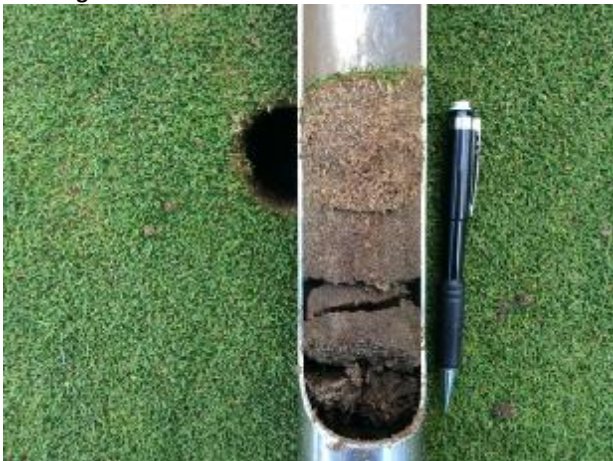
Figure 3: This was typical of soil conditions seen. There remains more organic matter in the upper 50 mm than ideal – this will hold onto moisture for longer promoting softer surfaces following rain/irrigation.
