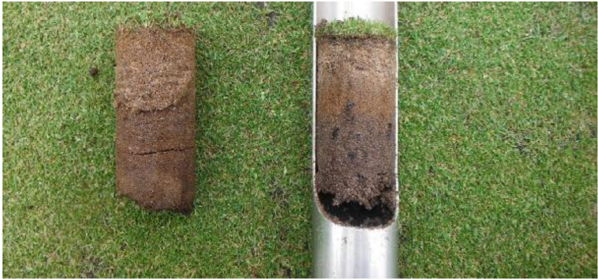
Cores from the original green (left) and new construction (right)
